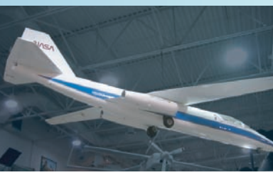
The NASA "Swing Wing" aircraft tests designs that allow an airplane to fly both slow and ultra-fast.
